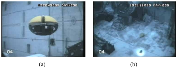
Fig. 9. A profiling operation, captured by under-water cameras at the Neutral Buoyancy Lab (NBL) at Johnson Space Center. Initially, the sonde is stowed in the vehicle. (a) During profiling, the sonde is smoothly spooled down. (b) When the sonde reaches a height of 1 m above the floor, a camera takes images of the floor.
