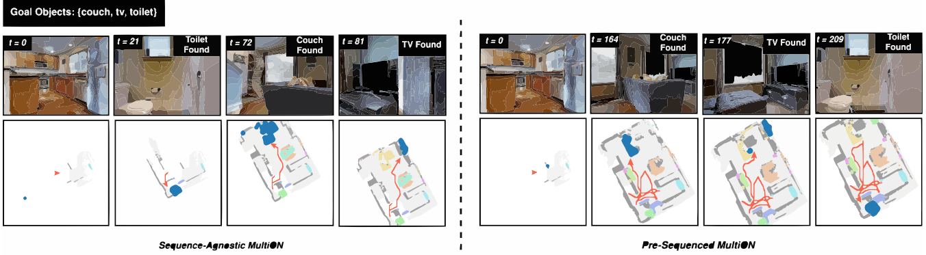
Fig. 3: Qualitative comparison of the performance of our SAM framework (left) with PSM (right) in an episode of the MultiON task with three target object classes (couch, tv, toilet). Our framework results in a smaller number of steps.
