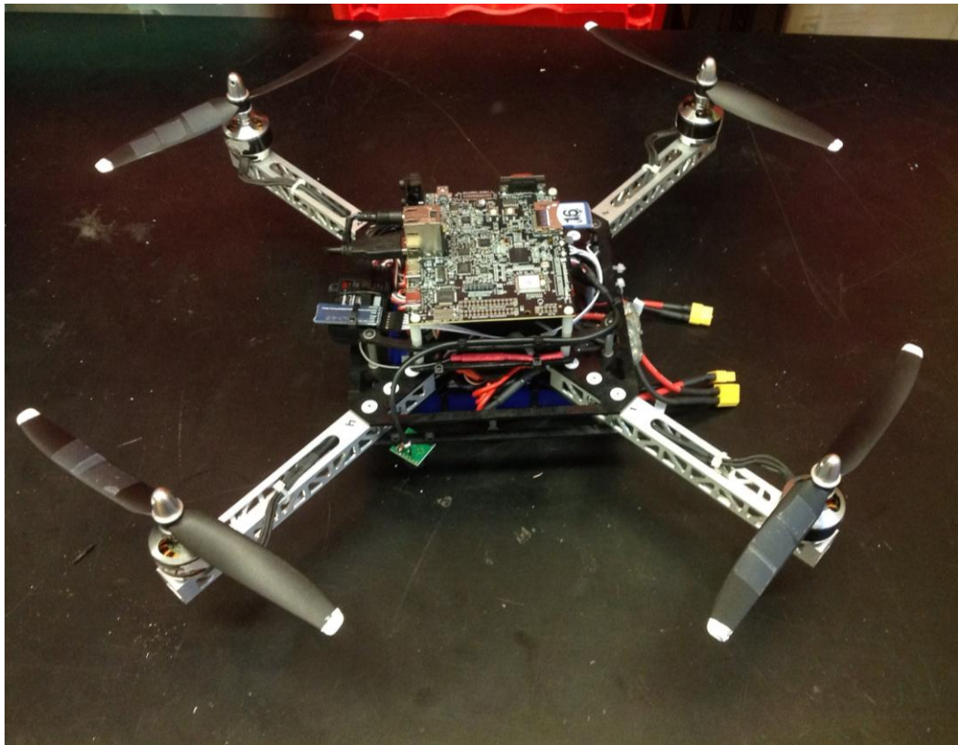
Figure 86: Quadrotor Airframe and Electronics
