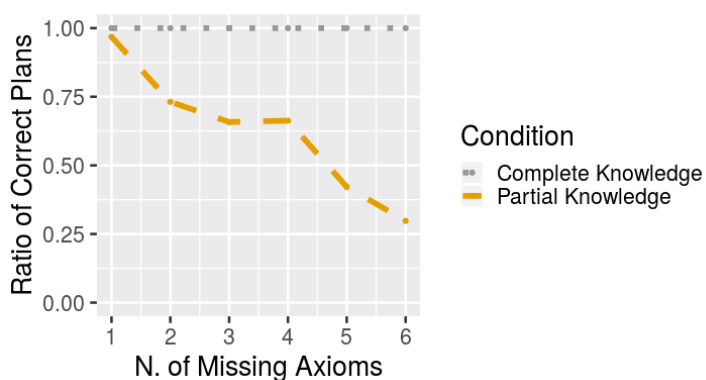
Figure 5: Ratio of correct plans out of all plans generated with increasing numbers of missing executability conditions 1-6.
