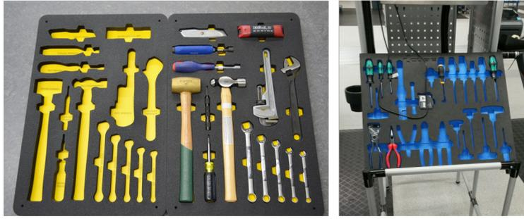
Figure 3: Example’s of shadow boards
