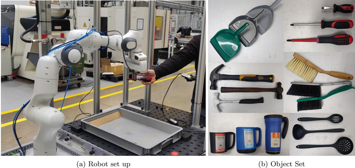
Figure 18: Franka manipulator robot and some objects used in the experiments. Where to grasp an object is dependent on task-specific and object-specific constraints in addition to stability.
