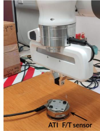
**Fig. B.14** Task setup for comparing external FT sensor measurements with the robot’s internal estimator.
