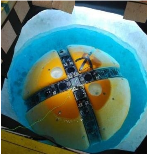
Figure 1: ENDURANCE AUV being deployed through the melthole in West Lake Bonney. The melthole diameter ( \approx 2 m) is only slightly larger than the vehicle's diameter ( \approx 1.8 m). A blinking light source was suspended approximately 1.5 m above the melthole.
