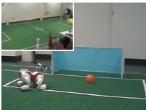
Figure 1: Aibo and field. The experiments reported in this paper are run on the SONY ERS-7 Aibo, a four-legged robot with a CMOS color camera with a limited field-of-view ( 56.9^\circ horz., 45.2^\circ vert.). The images are captured at 30Hz with a resolution of 208 \times 160 pixels. The robot has three degrees-of-freedom in each leg, and three in its head. All processing for vision, localization, motion and strategy is done on-board a 576MHz processor. The Aibos are used in the RoboCup Legged League, a research initiative where teams of four robots play a game of soccer on an indoor field (Figure 1).
