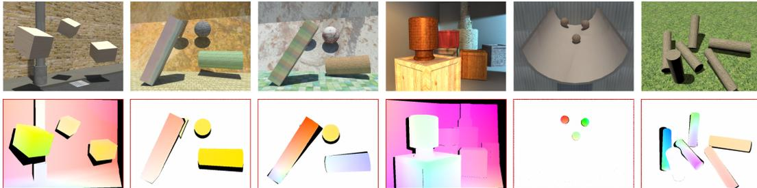
**Figure 4.2: Ground Truth Optical Flow Data** The top row depicts some example images from our system. Below is the ground truth flow between successive frames. The flow field color is coded using the same format as [9]. Black values in the flow image indicate areas of occlusion between the two frames.
