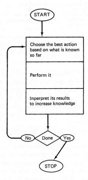
Fig. 10.20 A main executive control loop for heterarchical vision.
