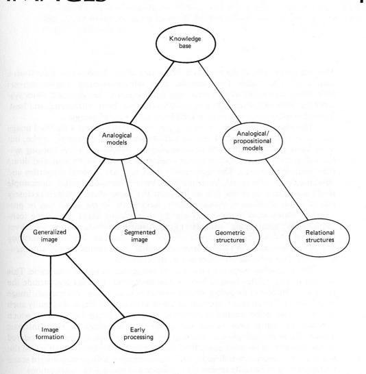
The first step in the vision process is image formation. Images may arise from a variety of technologies. For example, most television-based systems convert reflected light intensity into an electronic signal which is then digitized; other systems use more exotic radiations, such as x-rays, laser light, ultrasound, and heat. The net result is usually an array of samples of some kind of energy.
