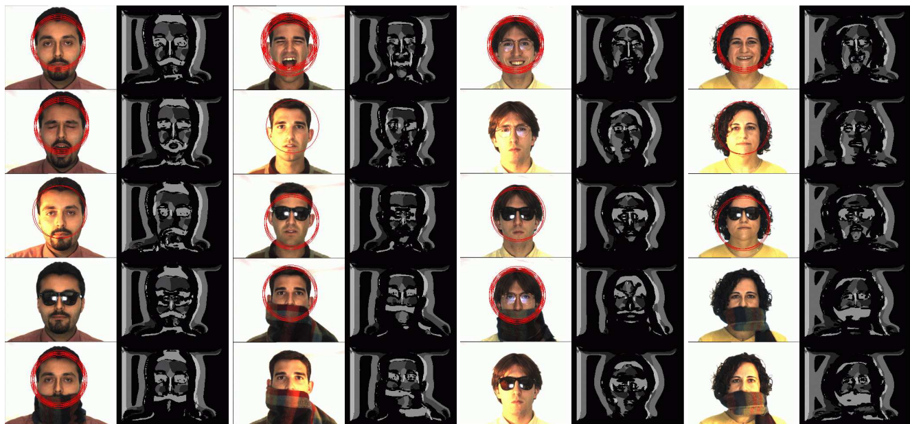
Figure 8: Classton channels of images under significant illumination changes. The classtons are obtained from 15 frontal faces under uniform lighting such as the image in the top row. The facial features are detected reliably. Face detection is successful in images with various facial expressions, strong illumination, and occlusions. It fails in cases with combined strong illumination and occlusions.
