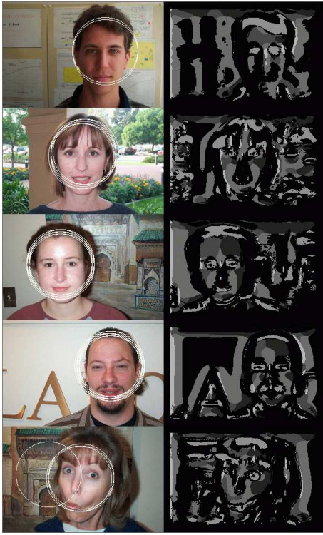
Figure 7: Classton channels of individuals other than the 15 neutral male training faces. All faces are reliably detected using a log-polar histogram, insertions due to background clutter are rare.
