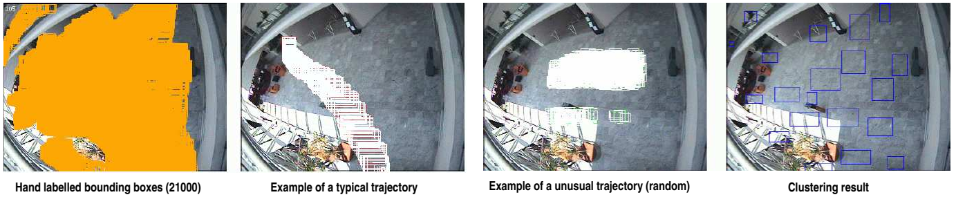
Fig. 4. Ground truth labelling for the entrance hall scenario, examples of typical and unusual trajectories and clustering result using k-means with pruning.
