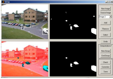
Figure 1. User interface used to create the ground truth from automatic segmentation results.
