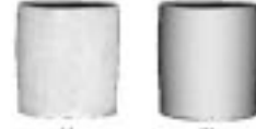
(a) is a photograph of a clay mug, while (b) is a Lambertian rendering from Oren & Nayar, "Generalization of the Lambertian Model and Implications for Machine Vision," IJCV , 14(3):227-251, 1995.
