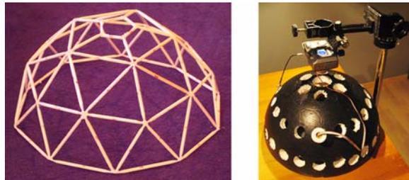
**Figure 8:** Two inexpensive domes useful for specifying lighting direction. In both cases a digital camera is placed above and the object to be imaged placed on the floor below. Right image courtesy of Wouter Verhesen.
