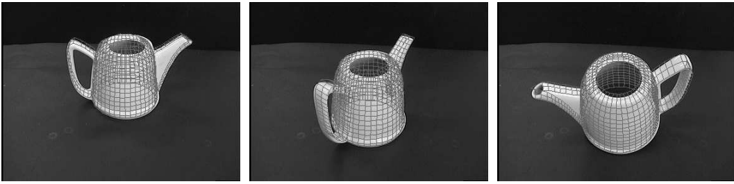
Figure 16: First pose results of the tea pot. The projected object model visualizes the quality of the 3D pose.
