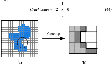
**Figure 9**: (a) Object including part to be studied. (b) Conto ur pixels as used in the chain code are diagonally shaded. The "crack" is shown with the thick black line.
