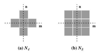
Figure 38: The standard structuring elements  $N_4$  and  $N_8$ .
