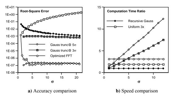
**Figure 28**: Comparison of various Gaussian algorithms with N=256. The legend is spread across both graphs
