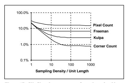
**Figure 17**: CV of length measurement for various algorithms.
