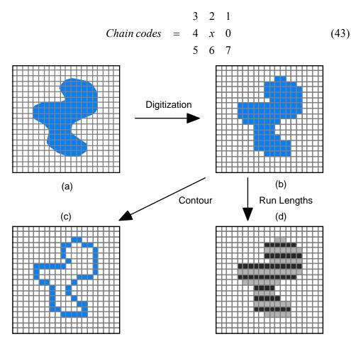
**Figure 8**: Region (shaded) as it is transformed from (a) continuous to (b) discrete form and then considered as a (c) contour or (d) run lengths illustrated in alternating colors.
