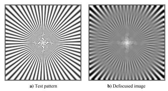
**Figure 23**: Convolution of test pattern with a pill box of radius a=4.5 pixels.
