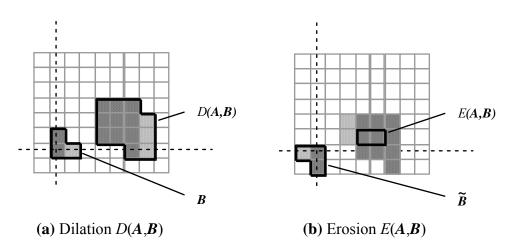
**Figure 37:** A binary image containing two object sets A and B. The three pixels in B are "color-coded" as is their effect in the result.
