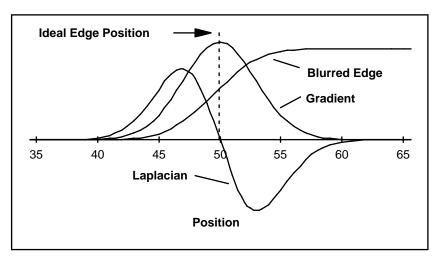
**Figure 54**: Edge finding based on the zero crossing as determined by the second derivative, the Laplacian. The curves are not to scale.
