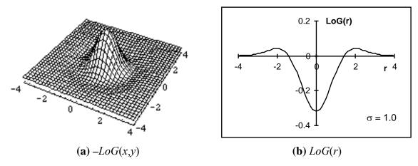
**Figure 55**: LoG filter with  $\sigma = 1.0$ .
