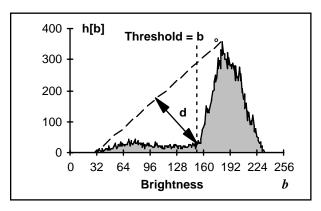
**Figure 52**: The triangle algorithm is based on finding the value of b that gives the maximum distance  $\mathbf{d}$ .
