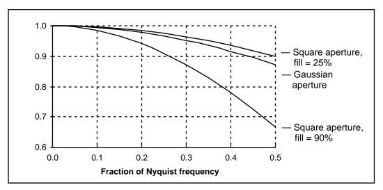
**Figure 16**: Aperture spectra P(u,v=0) for frequencies up to half the Nyquist frequency. For explanation of "fill" see text.
