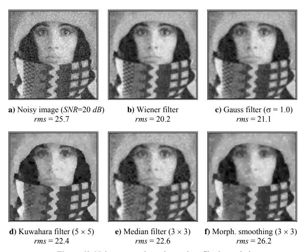
Figure 49: Noise suppression using various filtering techniques.
