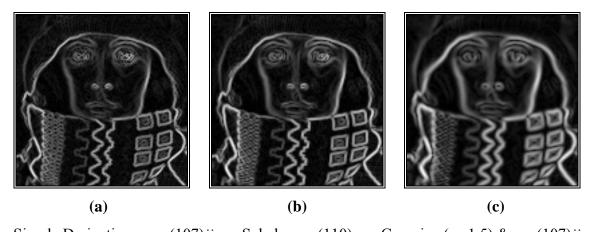
Simple Derivative – eq. (107)ii Sobel – eq. (110) Gaussian ( $\sigma$ =1.5) & eq. (107)ii
