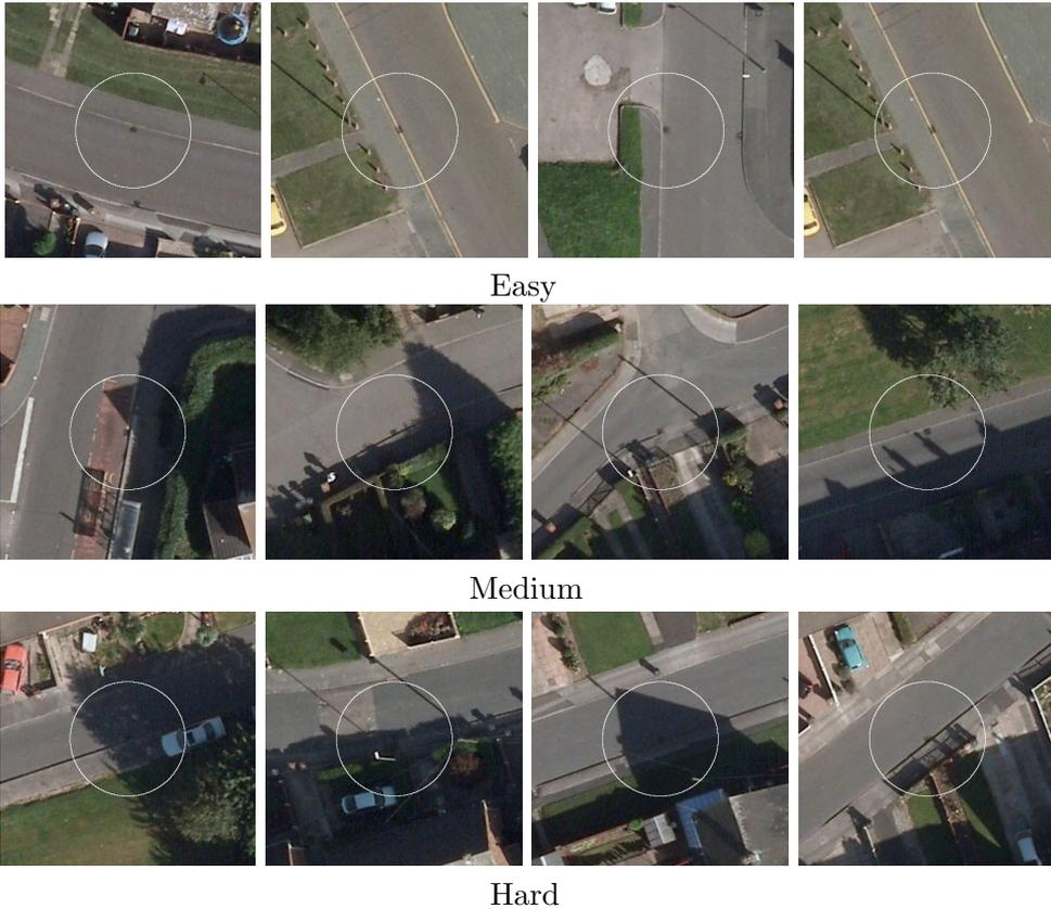
Figure 1: Examples of drains categorized by the difficulty of detection. The ‘Easy’ set presents no shadows or objects that could potentially obstruct detection and the road edge is characterized by a fairly straight line. In the ‘Medium’ set, the drain is still visible, although shadows might be present or the road edge not straight. The drains in the final, ‘Hard’ set are either covered by shadows or are considerably hard to distinguish from their surroundings.
