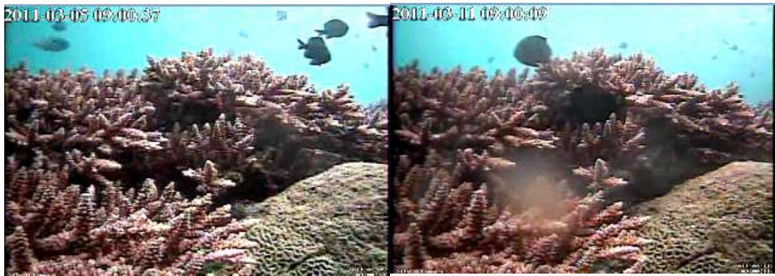
Figure 1.3: Frames taken a) with recently cleaned lens b) lens with particles and dirt on.
