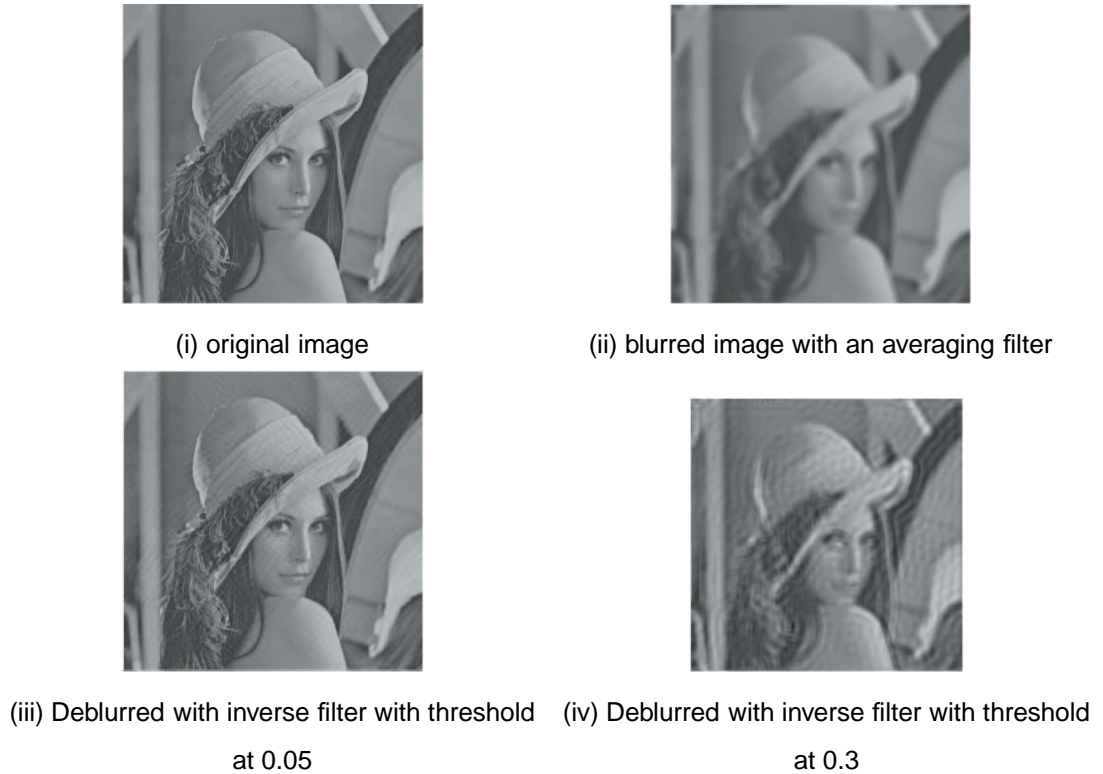
Figure 2.12: The effect the lower bound has on the reconstruction of inverse filtering.
