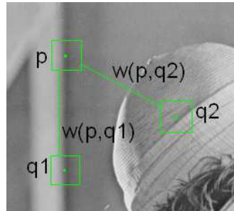
Figure 2.9: Example showing how patch similarity affects the weighting of the average. Weighting of q_1 will be larger than that of q_2 due to its patch's similarity with the reference patch. Image taken from [4]
