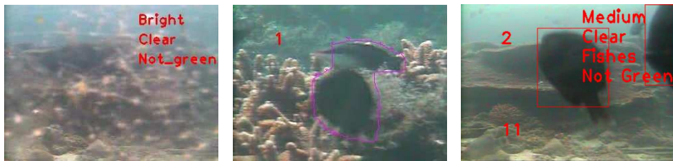
(a) T1: Video classification. (b) T2: Fish detection and counting in frames. (c) T1 & T3: Video classification, fish detection and tracking.
