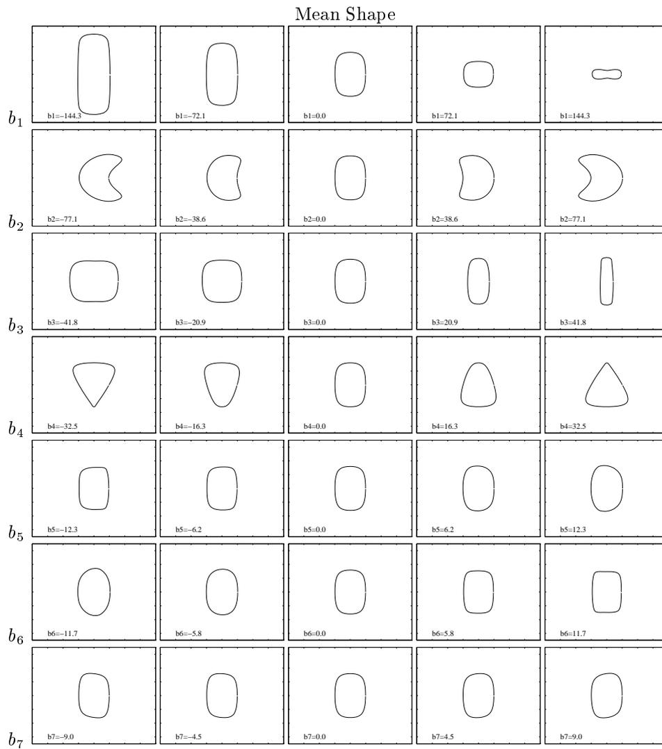
Figure 5: Parametrisation of the PDM model. The modes of variation controls the actual PDM shape in a rather neat way: the first four modes straightly control vertical height, bending, width and tapering, respectively, whereas the last three produce, in combination and unexpectedly, slight horizontal tapering, squaring and shearing.
