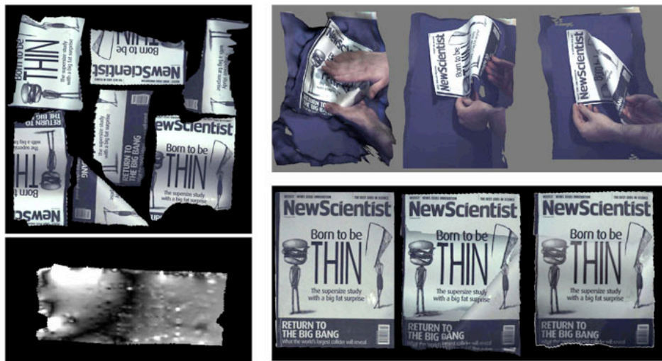
Figure 2: Deformable surface reconstruction from multiple range observations. TL: Regions matched and extracted from several range images (some of which are shown in TR). BL the resulting reconstruction comparing (left) the true surface texture, (middle) rigidly aligned patches and (right) the nonrigidly aligned and stitched model. BL: An example distortion map for a particular segment.
