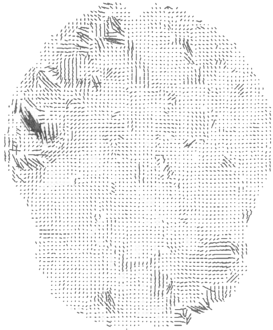
Figure 4.1: The residual vector map, showing likely local structure changes between images, computed as follows: A bi-variate cross-correlation local image region matching function is used on the images shown in Figure 2.1 to compute an initial image match map (Figure 3.3 (b)). This initial map is computed to sub-pixel level at a scale of four. Lone bad vectors are identified and removed (Figure 3.7 (a)). Finally global image transformation is estimated and removed (above). Plate 1 shows this image in full colour.
