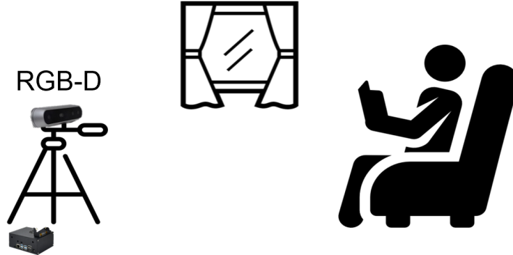
Figure 1: Real-time system for monitoring older adults in common home scenarios (inactivity monitoring of routine seating areas). Anonymous monitoring uses a compact system consisting of an RGB-D camera and a small computer processor. Anonymity is maintained by discarding captured images after processing.
