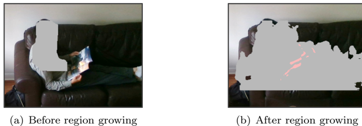
Figure 3: A person sitting on a couch. The grey area shows the foreground detected using the depth map (a) before the region growing and (b) after the region growing. Real human motion (red) is not detected in the incomplete foreground before the region growing.
