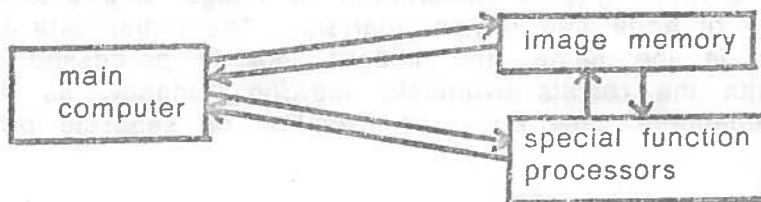
Figure 7 - Functionally Parallel System Structure (Each unit executes in parallel with others)
