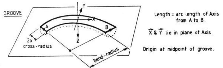
Figure 6: Definition of GROOVE Feature
