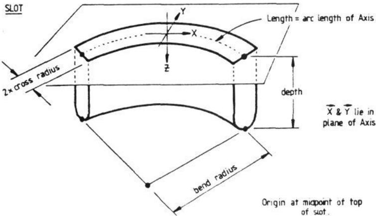
Figure 7: Definition of **SLOT** Feature
