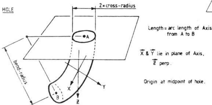
Figure 5: Definition of HOLE Feature
