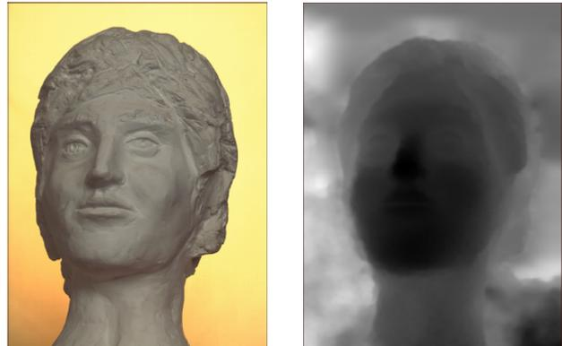
and here are two views of the surface reconstructed from the fusion of 220 views:
