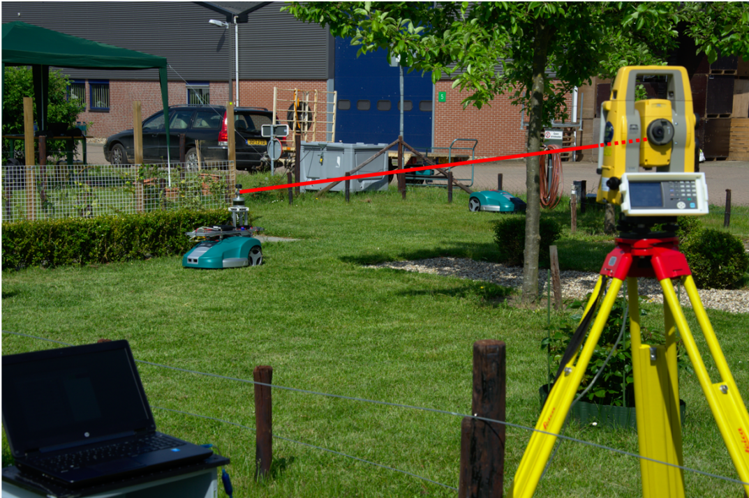
Figure D.2: Topcon PS Series Robotic Total Station estimated the robot’s 3D position by emitting laser beams and receiving the beams reflected by the prism reflector on the top of the trimming robot Trimbot.
