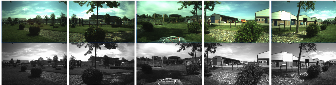
(c) 10 synchronized images from the panoramic stereo camera consisting of 5 stereo vision cameras (10 image sensors in total)
