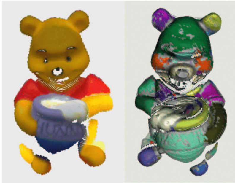
Figure 2: Part decomposition - range image (left), decomposed parts represented by different colors (right) with \alpha = 0.1 , \beta_1 = 0.01 and \beta_2 = 0.01 .
