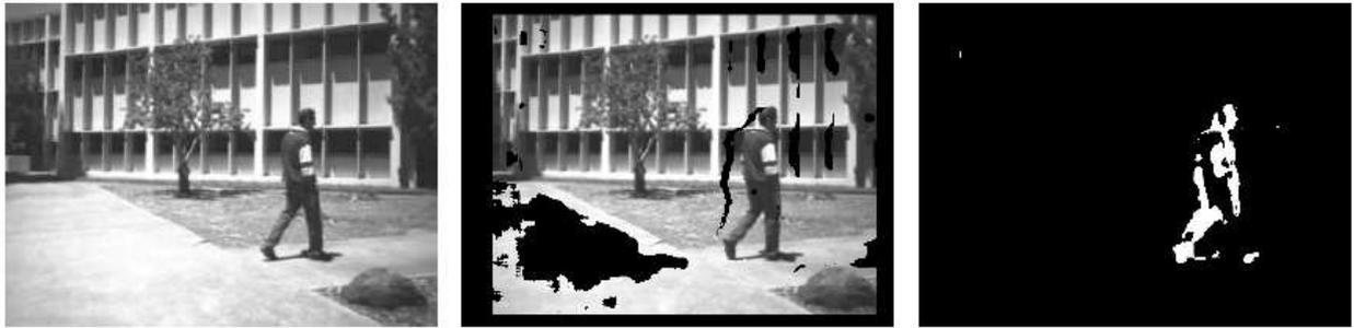
Figure 22.19: Independent motion detection from a moving platform. Reference image on left is forward-projected using the motion homography to the center image; right image is difference with actual image.
