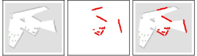
Figure 22.15: Scan match by maximum likelihood against several reference scans in an occupancy grid.
