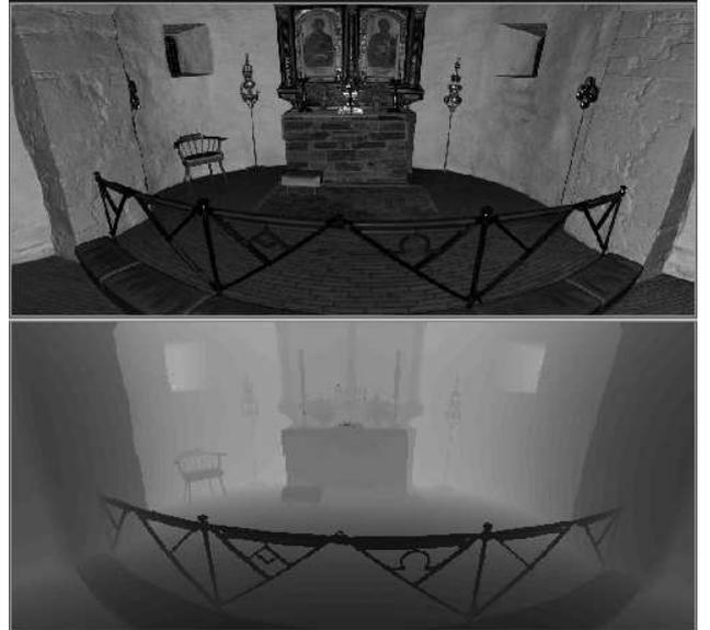
Figure 22.1: Above: Registered infrared reflectance image. Below: Range image where closer is darker.
