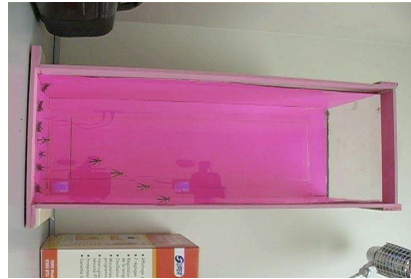
Figure 3: Experimental setup for grasshopper monitoring. A “time-lapse” visualization of a portion of video is used – only one grasshopper is present in the enclosure. A stereo pair of cameras is used, only one image is shown here.
