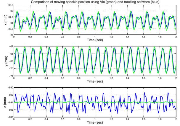
Fig. 3. Comparison of position trajectory of a fiducial pattern on the artificial spring mass body using the VIC (green) and tracking software (blue).
