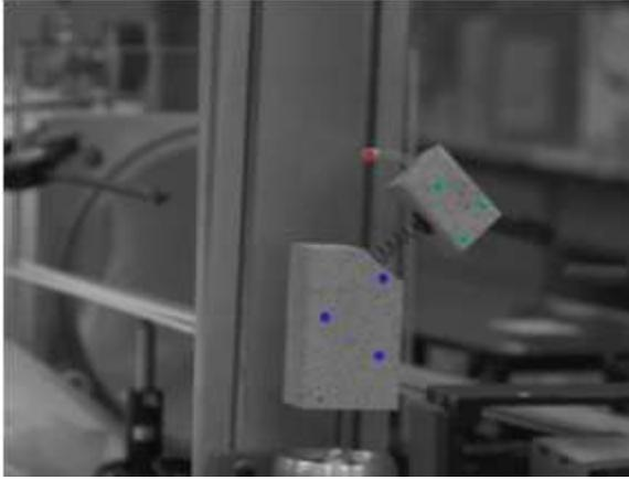
Fig. 2. The artificial target, with points tracked on the body (blue), head (green) and antenna (red).
