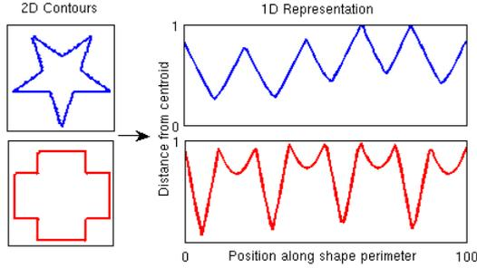
**Figure 2. Representation of 2D contours using 1D signatures (see text for details.)**
