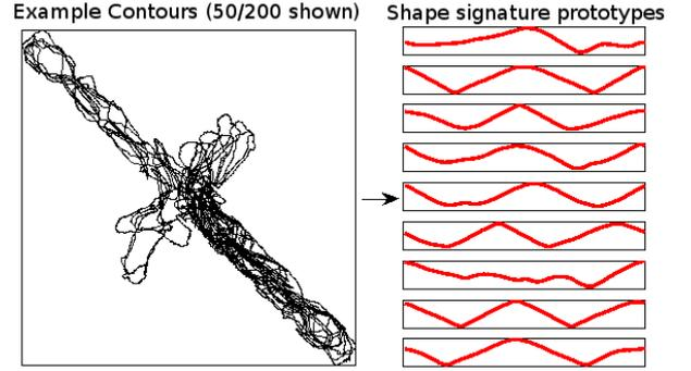
**Figure 4. Extraction of shape signature prototypes from a set of example contours (see text for details.)**
