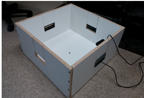
Fig. 1. Custom cage with camera nests.
