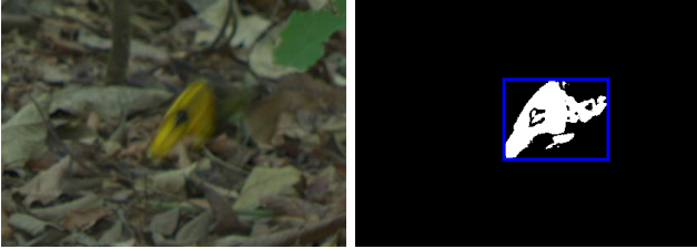
Figure 3: Foreground mask (right) generated by MOG model of frame (left). Blue box: extracted blob.
