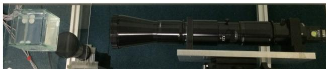
Fig. 1. One axis of the imaging setup including a telecentric lens pointing at a fluid-filled cube.
