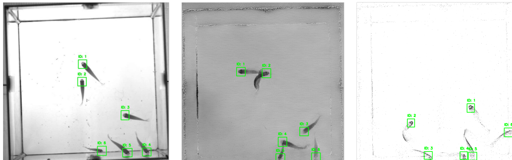
Fig. 1: Visualization of the tracking output on different sensor data. From left to right: tracking on grayscale frames of a conventional camera, on images reconstructed from event data using E2VID [1] and on time maps obtained from event data.
