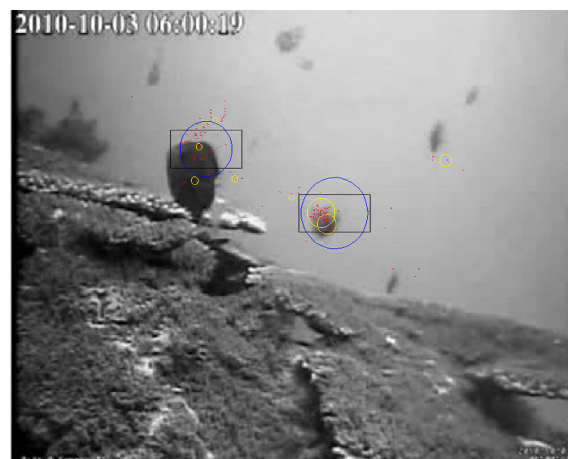
Figure 8: Clustering applied on the acquired data: Red dots are the locations clicked by the users. Yellow circles represent the result of the first clustering iteration, while the blue circles are the final result of the clustering method. The radius of each circle is equal to the sum of the quality scores of the users that made an annotation that belongs to that cluster, given by (3).
