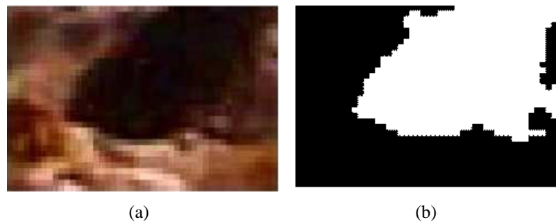
Figure 3: a) Original Image with low contrast fish/background, b) Output of the detection task enhanced with segmentation carried out with the simple region growing algorithm
