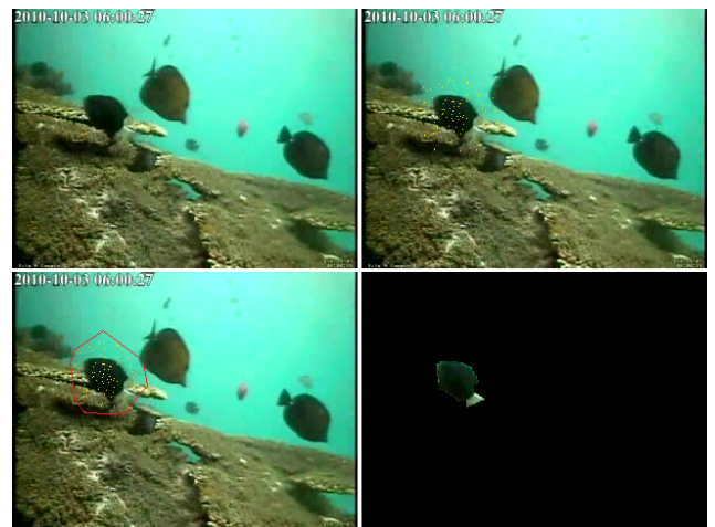
Figure 5: Example of the application of the Grabcut segmentation algorithm. On the top left the original image can be seen, while in the top right the points that belong to an identified cluster are shown in yellow. The convex hull of these points is calculated ( bottom left , in red) and Grabcut is applied on it ( bottom right ).
