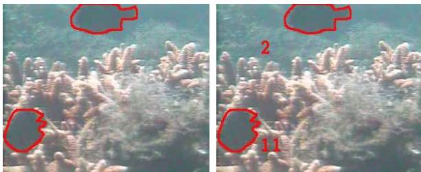
Fig. 4. Example tracking level processing for fish counting in a video. Sample results for fish detection (left) and fish counting (right). The top number indicates the number of fish in the current frame and the bottom number indicates the total number of fish in the video so far.
