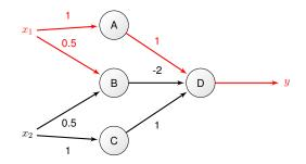
(neurons arranged in layers, and fire if input is  $\geq 1$ )
