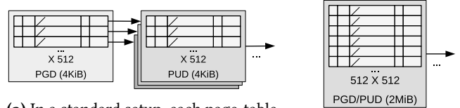
(a) In a standard setup, each page-table level is stored across 4 KiB frames, holds 512 elements, and thus translates 9 bits of the virtual address. One memory access is required to look up each level.
