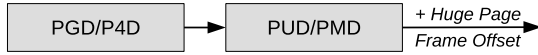
(c) If most PMD entries down a path are to huge pages, then all levels can be made dense even with an odd number of layers.
