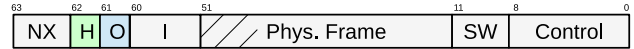
Figure 7. We add two bits within the ignored region [1] of our radix-tree layers: the first, H, indicates that we are pointing to a merged 2 MiB frame. The second, O, is used to denote overlap, to improve caching (section 4.3).
