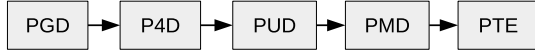
(a) Five-level page tables introduce a new layer, P4D, to increase virtual-address size from 48 to 57 bits.
