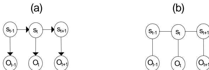
Figure 5.1: (a) an HMM, (b) an analogous linear chain CRF for phone representation.
