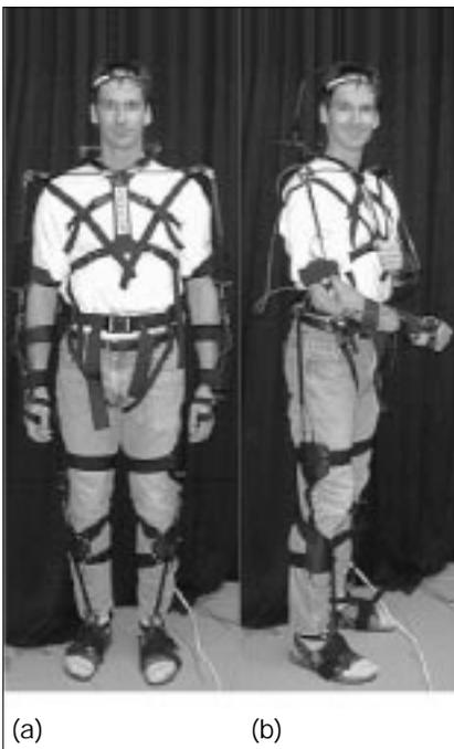
Figure 12. The Sensuit motion-capture system.
