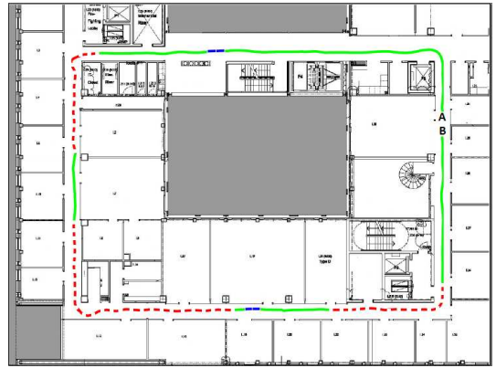
Fig. 5. Test 1: Robot path configurations (AMCL on Laptop [green], AMCL/AR on Robot [red], AMCL/AR on Laptop [blue]).
