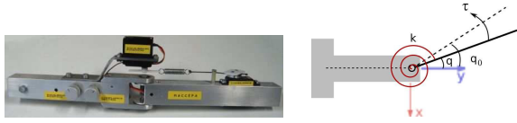
Fig. 3. MACCEPA VIA [4] and simplified dynamics model (image taken from http://mech.vub.ac.be/multibody/topics/maccepa.htm ).
