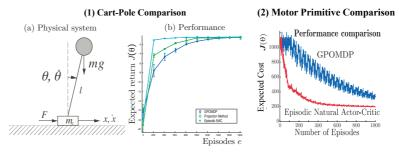
**Fig. 2.** This figure shows two comparisons, (1) cart-pole and (2) motor primitive learning. The physical set-up of a cart-pole balancing is shown in (1.a), and in (1.b) the performance of GPOMDP, the projection natural gradient, and the Episodic Natural Actor-Critic in comparison. The latter clearly outperforms the first two.
