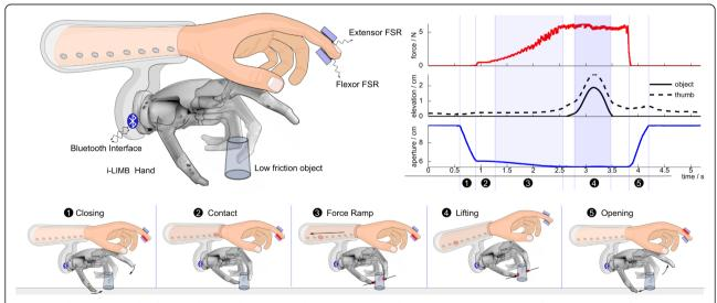
**Figure 1 The 'Grasp and Lift' paradigm with our Closed-Loop prosthetic hand**. Healthy subjects were fitted with a modified i-limb Pulse prosthetic hand with a two-channel differential force controller. Grip-force feedback was delivered to their arm using a vibrotactile feedback array (see *methods*). They were instructed to grasp, lift and replace a low-friction object (inset 1-5). A typical trajectory (showing grip force, object and thumb elevation, and grasp aperture) is also shown.
